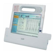
Docking station with USB and LAN connectors as well as battery charger
